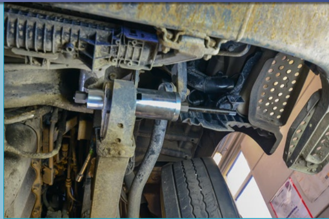
Pull out defective bush
