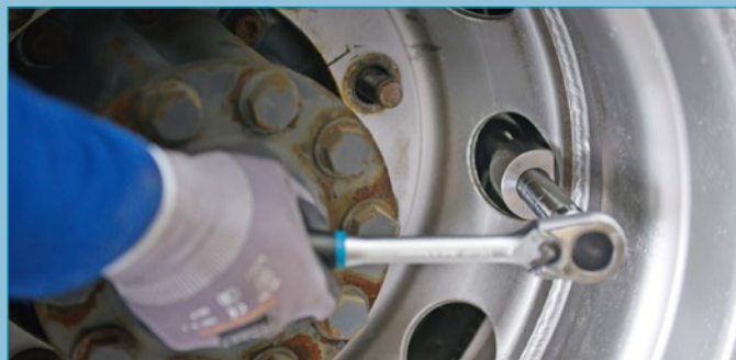
Rotate the spindle drive size 17 until the outside rim disengages from the inner rim
