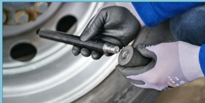
Place the rim flange support on the socket at the end of the spindle
