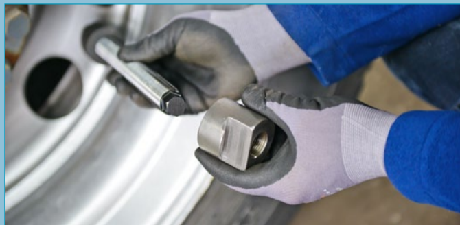
Select one of the two thrust blocks (abutment) depending on the rim's construction type and screw it onto the spindle
