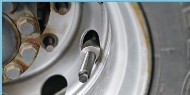
Now operate the spindle until the thrust block (abutment) lies against the inside of the rim hole
